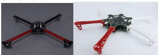
Fig. 2. Basic Quad and Hex Rotor frame Unmanned
